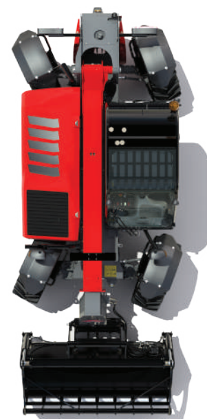
Four-wheel steering mode - for minimum turning circles.
