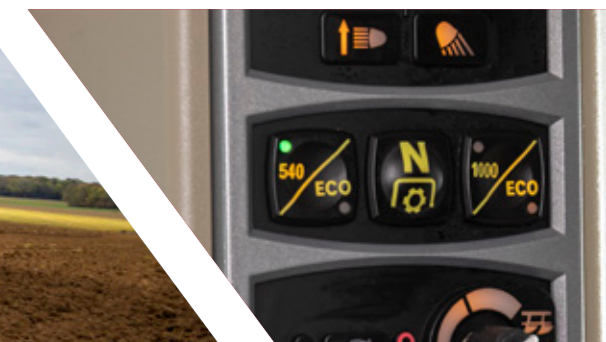
Electro-hydraulic PTO speed selection
