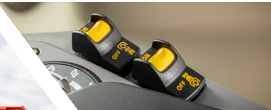
Electro-hydraulic PTO speed selection
