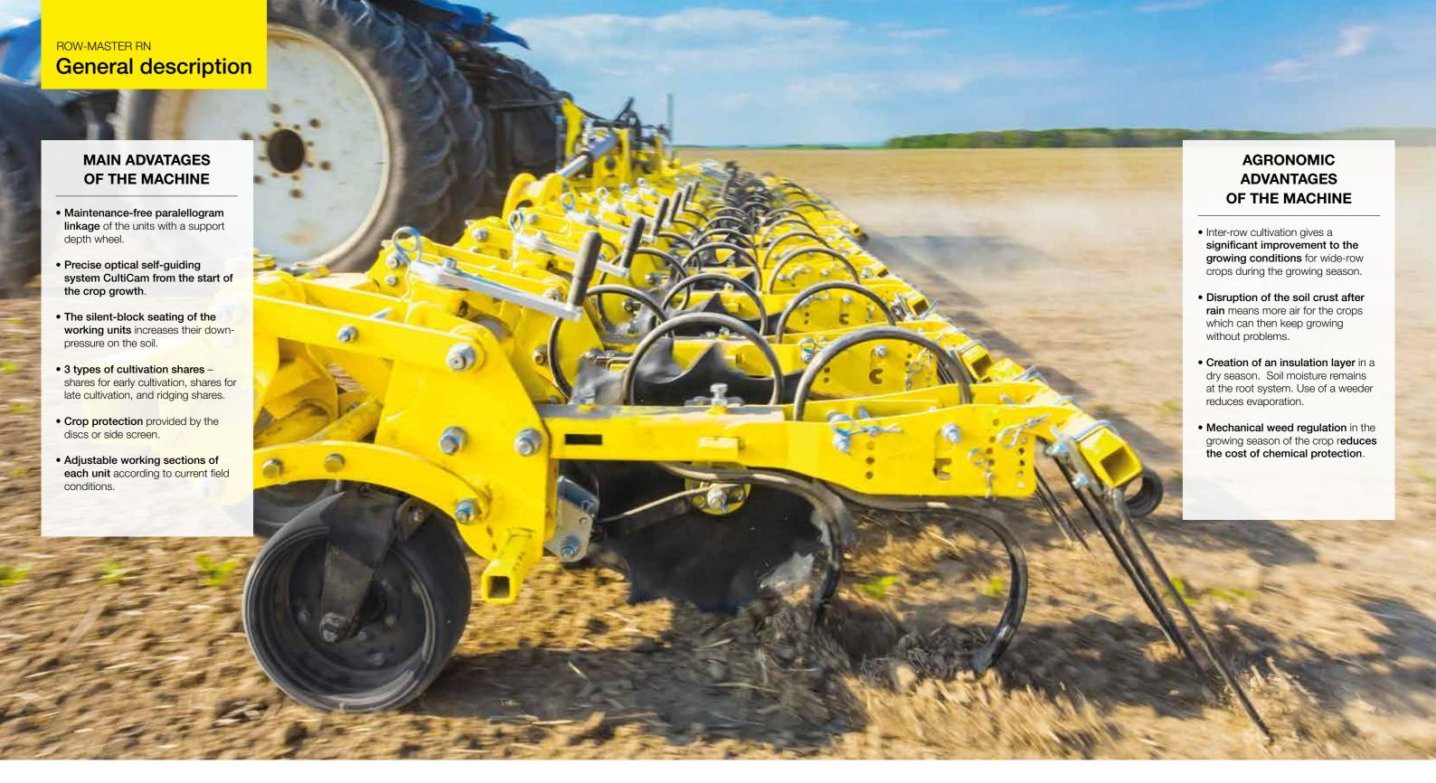
ROW-MASTER RN and RN\_S cultivators are designed for inter-row cultivation (disruption of the soil crust) and weed regulation in maize, sunflower (RN) and sugar beet (RN\_S) crops. The cultivators have variably adjustable working sections of each working unit so as to be able to react to current soil conditions and the size of the crops. Maintenance-free silent-block seating of the working units produces down-pressure on the support wheel and maintains a precise working track of each unit.
