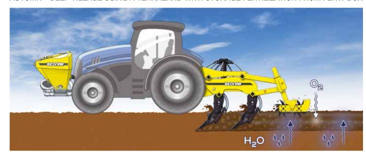
SPRING - SPRING PRE-SOWING PREPARATION USING A SWIFTER WITH SB SHARES
